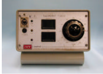
T3000 Achieved and Target temperature displays. The T3000B and T3000E looks similar
