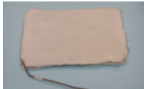
A view of a Heating Pad with the cover removed to show the padding. Note the serial number on the cable.
